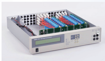
Figure 4. Vitrek's 964i offers automated multi-conductor, multi-point hipot testing.
